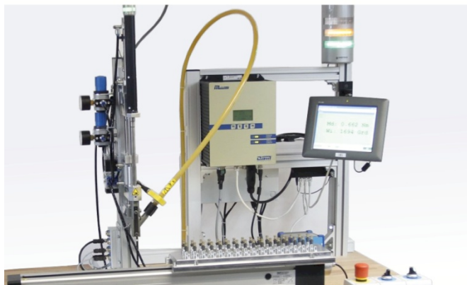
DSM assembly station for the automated tightening of thread nuts.
