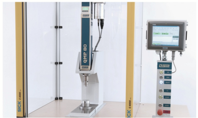
DSM press-fit station with protected working space for caulking of bushings.
